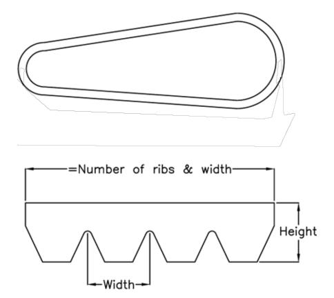
$\begin{array}{ll} \text{Datum Llength} = 1136 \\ \text{Height} &= 3.5 \\ \text{Number of ribs} = 18 \\ \text{Pitch} &= 2.34 \\ \end{array}$
